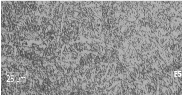
Figure 7. Weld metal microstructure of E5 (five passes weldment to St52 base metal with E electrode)
