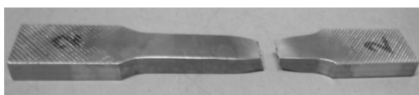
Figure 7. Tensile specimen of wire ruptured from base metal as a sample
