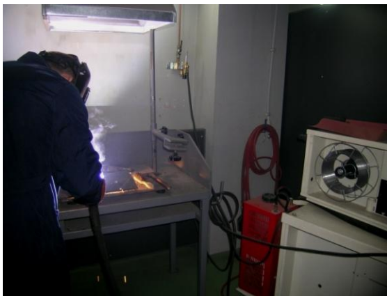
Figure 3. Experimental setup by using semi-automatic welding procedure
