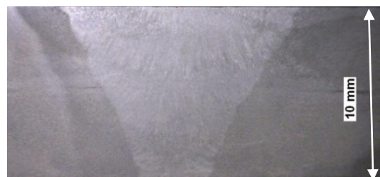
Figure 5. The cross-section of the weld joints i.e. G wire
