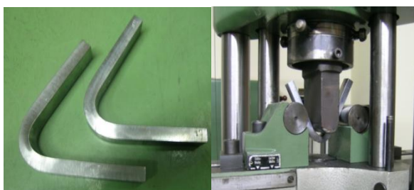
Figure 9a. Bending specimen image and bending test
